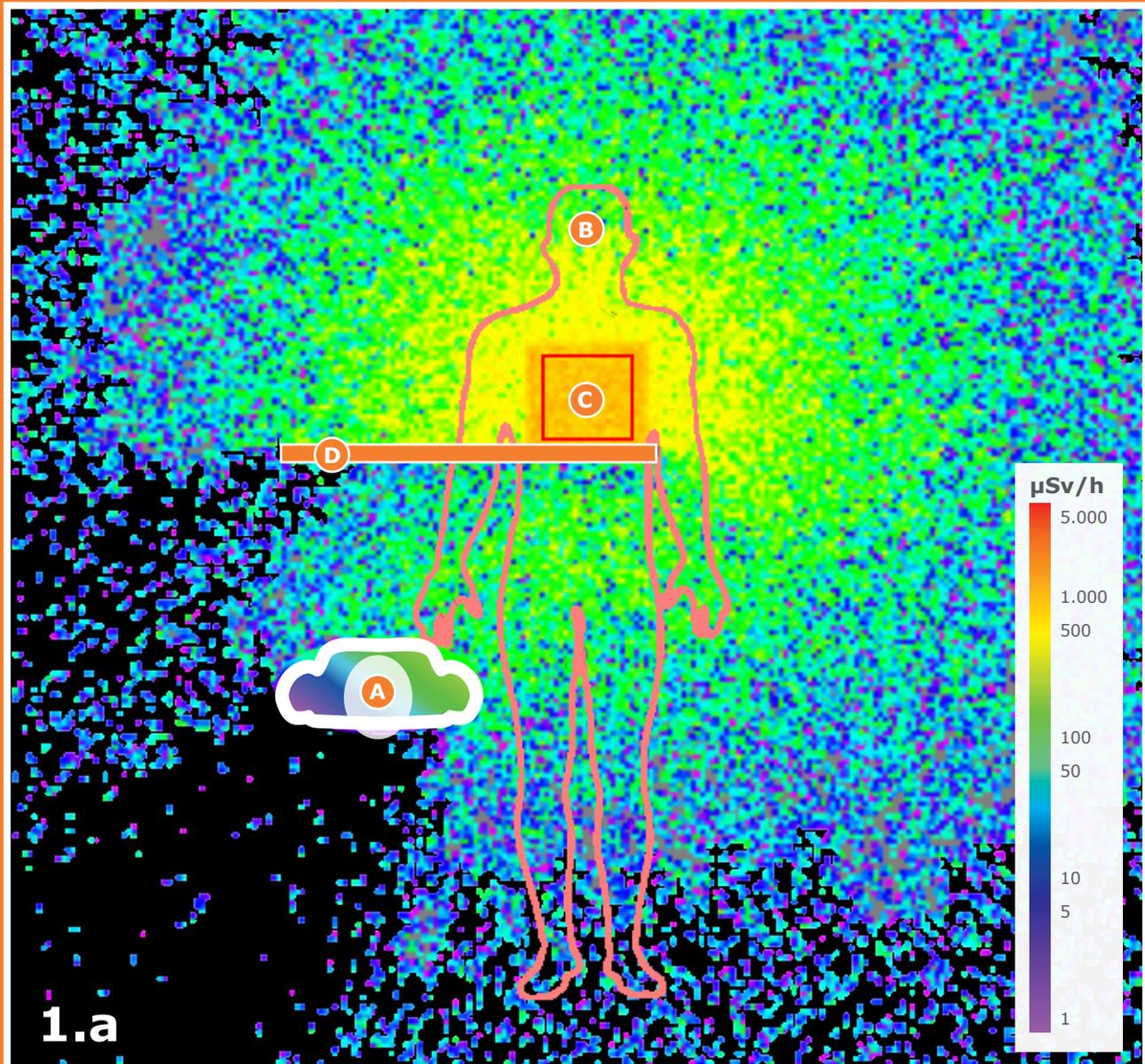
This Monte Carlo simulation allows a visualisation of the scattered radiation that passes through the patient's body and is released behind the shield. Figure 1.a shows the situation for the examiner when using a radiation protective shield without curtain.
