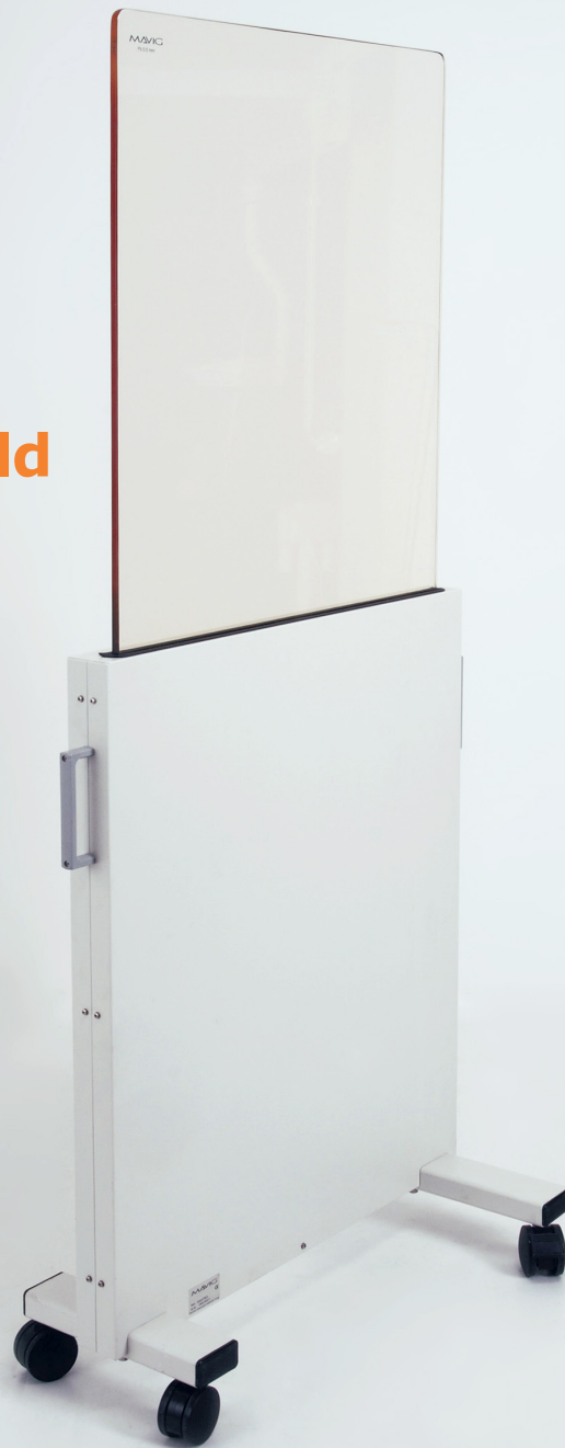
WD257 Mobile shield for versatile applications with a transparent and height-adjustable lead acrylic panel and a lead equivalent of: Steel body: 1.00 mm / Lead acrylic panel: 0.50 mm
